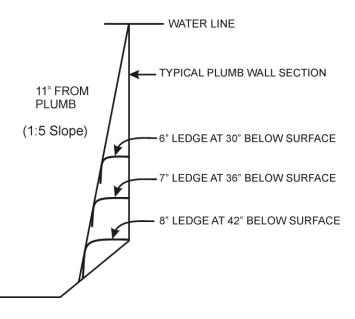
(9) **Underwater Seat Benches.** Underwater seat benches in pools, if provided, shall have a maximum horizontal seat bench depth of twenty inches below the waterline, be
