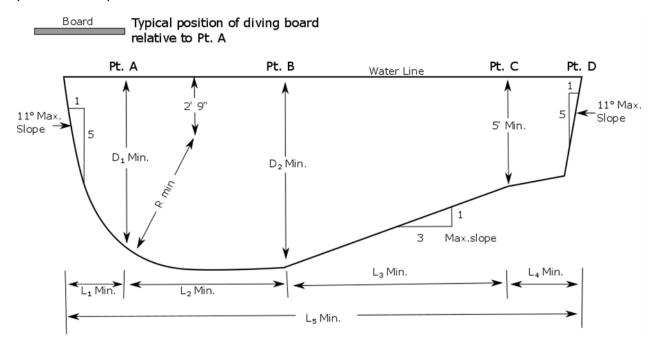
Note: L4 is a minimum dimension to allow sufficient length opposite the board. This may of course be lengthened to form the shallow portion of the pool.
